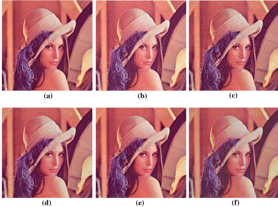
Fig. 9 Different noises added into the Lenna image. (a) Lenna image, (b) Gaussian noise with \sigma = 0.05 , (c) salt and pepper noise with \sigma = 0.05 , (d) speckle noise with \sigma = 0.05 , (e) Poisson noise and d periodic noise with amplitude A = 60 , angular frequency \omega = 30
