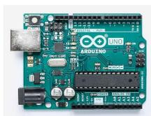
FIGURA B.1: Placa Arduino UNO
