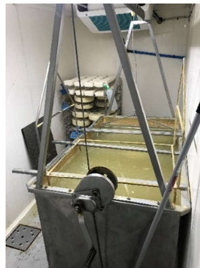
Figure 5.14: Salting process: Salting bath where the Ermesenda cheese wheels are submerged
