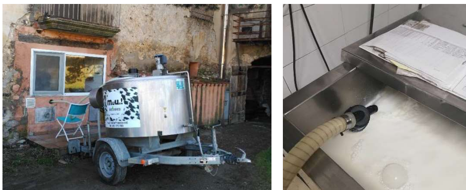
Figure 5.9: Raw milk reception and pumping process from the container trailer to the heated tank.
