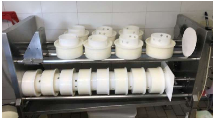
Figure 5.13: Cheese pressing process: Moulds with curds in the pressing machine
