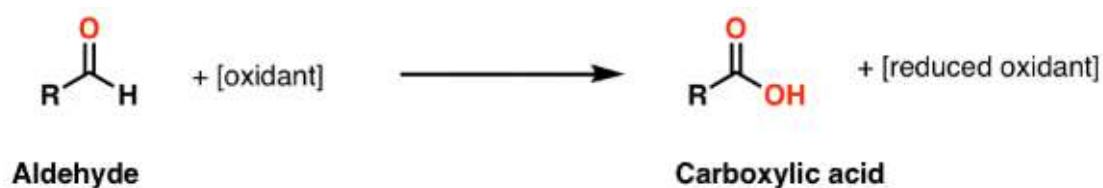
Figure 15. The aldehyde is oxidized to a carboxylic acid (break C-H, from C=O). The aldehyde reduces the oxidant. Therefore, the aldehyde is the reducing agent here. Source (26)
