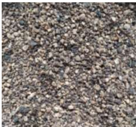
Figure 18. Olive-mill solid waste.
