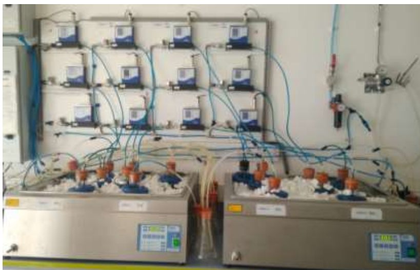
Figure 19. Bioreactors, where the solid-state fermentation to produce the enzymes, took place. They are connected to the respirometer to control the oxygen source and consumption.
