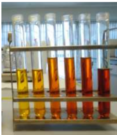
Figure 22. Bank of dilutions of glucose concentration used to DNS calibration curb. The intensity of the colour is proportional to the concentration of sugars.
