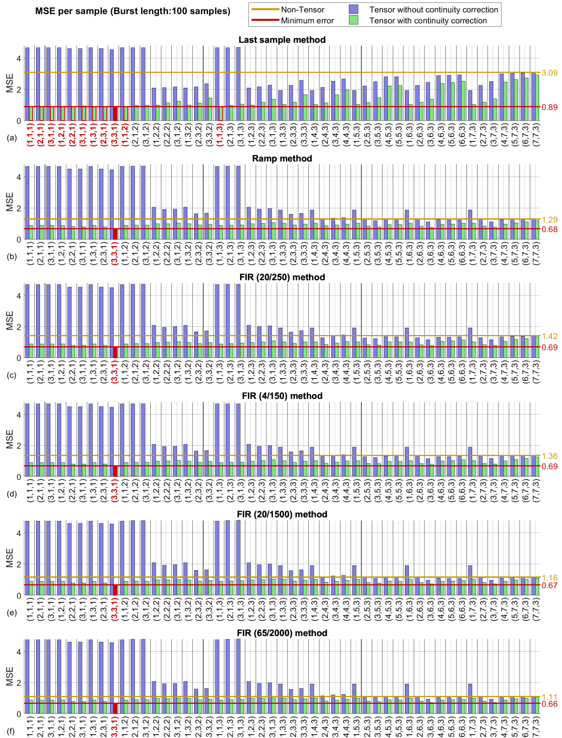
Figure 10. MSE per sample of the Tucker decomposition depending on the core tensor. The MSE of the restoration is shown with the continuity correction and without it. The bars marked in red have an error no bigger than 5% of the minimum.
