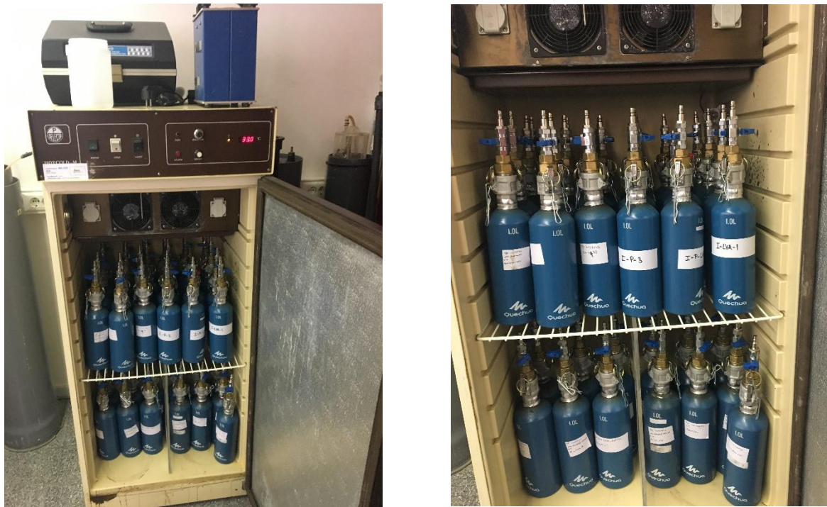
Figure 3. 7 Set up for anaerobic index determination: sealed aluminum bottles.
