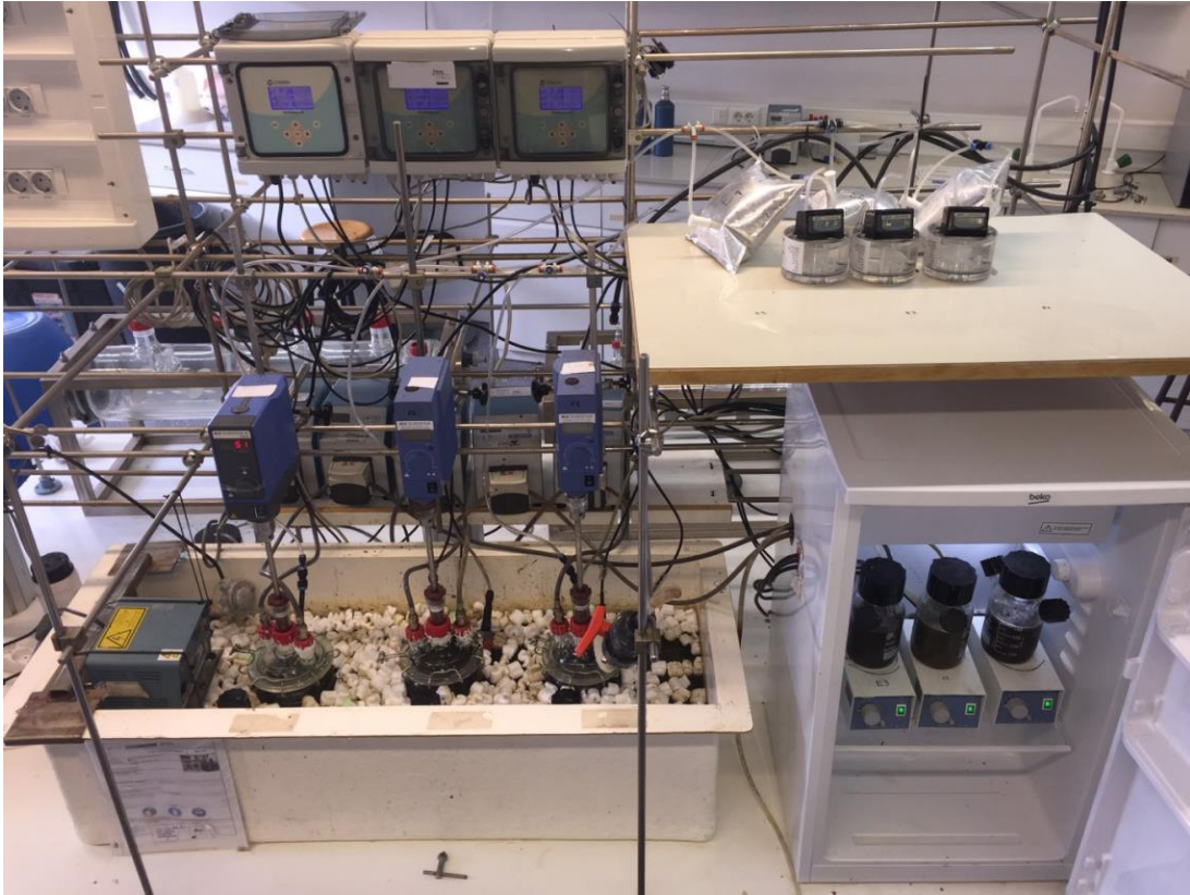
Figure 3. 13 Experiment set up for co-digestion of Cheese whey and animal manure
