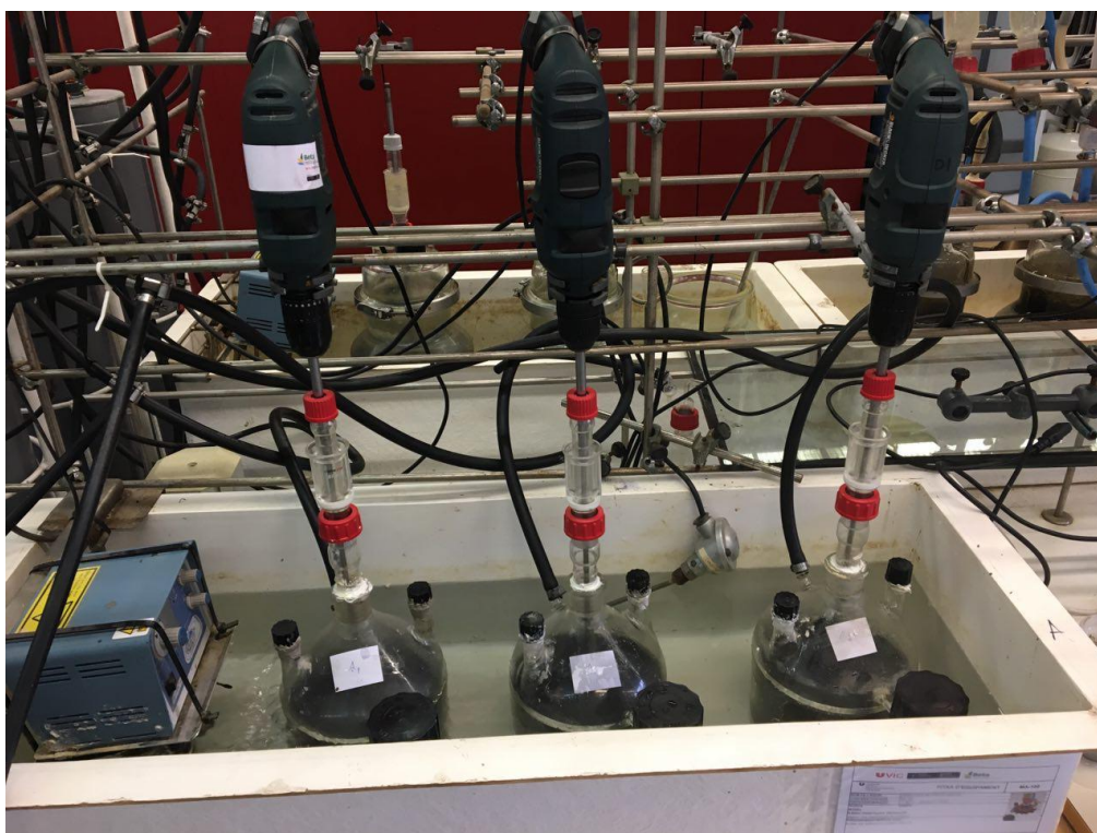
Figure 3. 10 Experiment setup of semi continuous reactors
