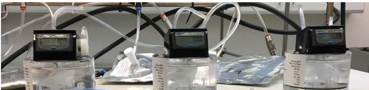
Figure 3. 14 Digital Gas meter
