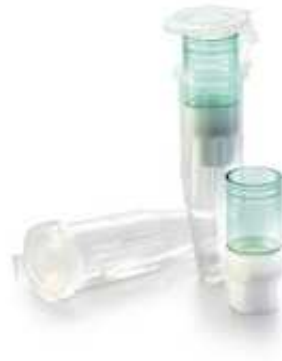
Figure 15: Microcon centrifugal filters used in the FASP protocol.
