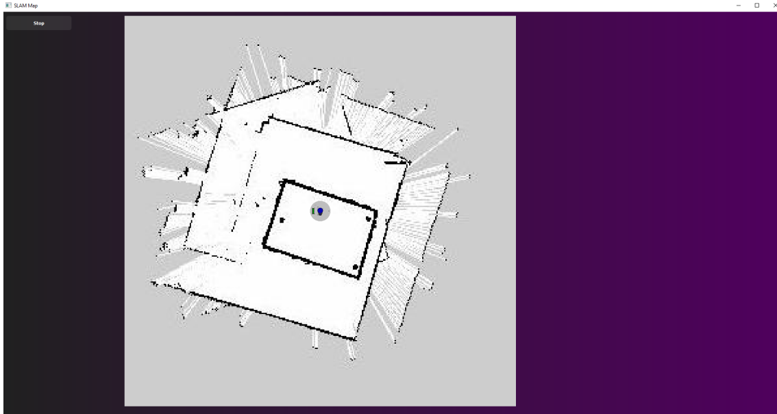
Figure 3.23: SLAM visualizer window where is represented the SLAM map that the robot computes.
