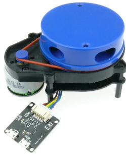
Figure 2.12: Lidar sensor model YDLidar X4.
