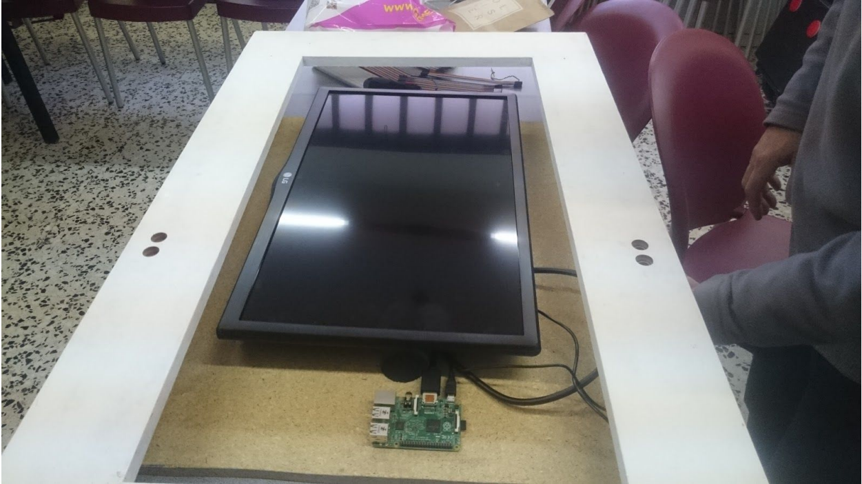
Appendix 6. Fully assembled device (only the glass panel missing)
